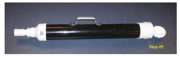
To complete assembly, add a garage door handle (part 14) to the top of telescope. Pick a handle that is constructed so that it is formed in a tube where you grasp it. Be careful to align it along the length of the telescope. The telescope tubes have writing imprinted along their length, which can be used to align the handle. With this type of handle and proper alignment, you will not only have a convenient way of carrying your telescope but a finder sight as well.
