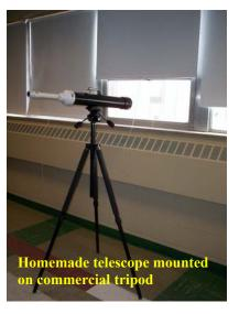
Step 1: One of the simplest focusing mechanisms is a draw-tube design. One can be constructed by using 1" diameter tubing about 12" in length (part 2) held in place by a short length (1" to 3") of 1-1/4
